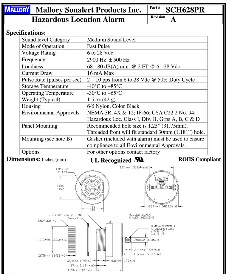
NDTE A: TERMINALS-.032 BRASS TIN PLATED, TAPPED FOR #6-32 SCREW. TWD #6-32 NICKEL PLATED BRASS SCREWS INCLUDED. WILL ACCEPT 1/4" QUICK CONNECT. NDTE B: MDUNTING- REMOVE BLACK PLASTIC NUT WHILE LEAVING GASKET ON THREADED NECK DF ALARM. INSERT THREADED NECK THRDUGH APPRIPRIATE SIZED PANEL HOLE. SCREW NUT BACK ONTO THREADED FRONT SECURING ALARM TO PANEL. MAX RECOMMENDED TURQUE IS 10 IN-LBS.
